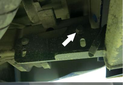
7. Mount bracket to the chassis using factory bolts from the bumper. Use adjusting bars.
