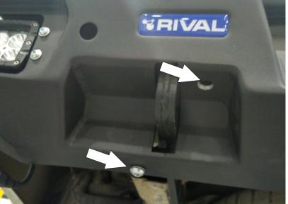
8. Mount bumper body to the bracket using screws M10x30 and washers 10.
