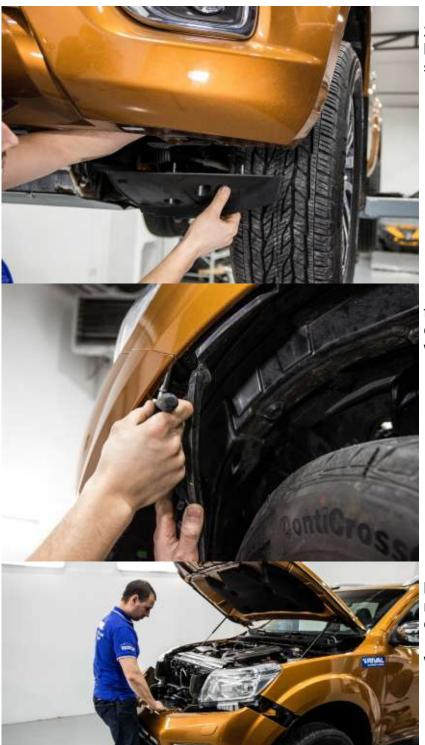
11. From the bumper inside, screw out 2 nuts which fasten the bumper skirt lateral part, and dismount the bumper skirt lateral part.
