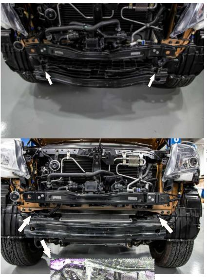
18. Remove clips which fasten the air intake. Dismount the air intake.
