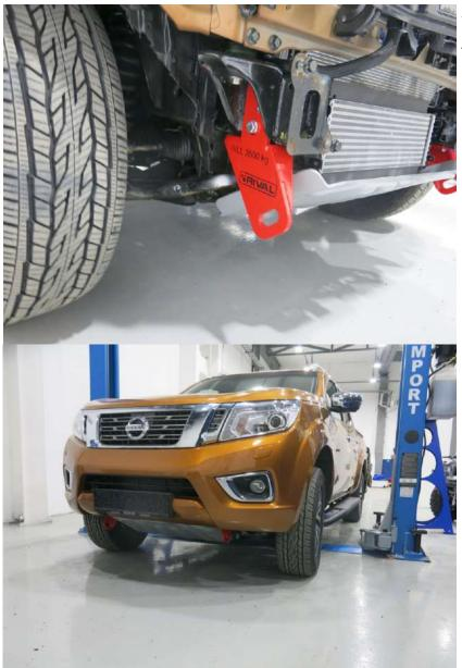
25. Fasten the towing loop (item 2) in lower part with standard bolts which fasten the towing eye.
