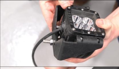
18. \*Mount lights (19) on brackets (4) using fittings from light set. \*For package with LED lights.
