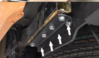
17. Mount bracket on reinforcement using bolts M10x40 and washers M10x20. Do not tighten yet.
