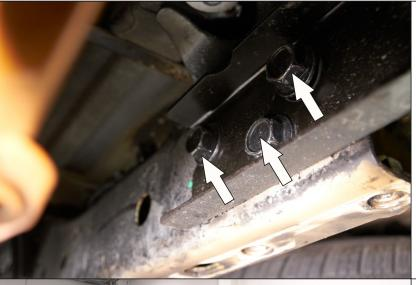
5. Unscrew 3 bolts of rear bumper mount from left and right side.
