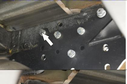
13. Mount bracket (2) on inside nut M10 (5) using bolt M10x40 (10) and washer M10x20 (16). Do not tighten yet.
