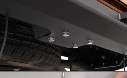
22. \*Mount bumper body (1) on bracket (2) in lower part using bolts M12x40(11) and washers M12x24(17). Tighten all screws.
