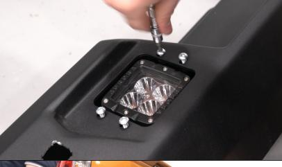
19. \* Mount brackets on bumper body (1) using screw M6x16(13). \* For package with LED lights.
