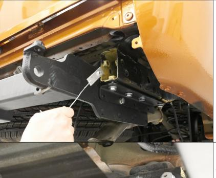
10. Mount inside nut M10(5) into the vehicle frame from the right side.
