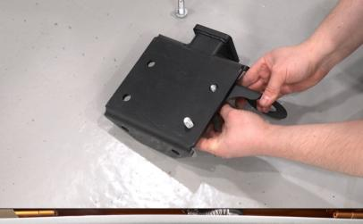
23. Mount socket bracket (9) on tow bar bracket (3).
