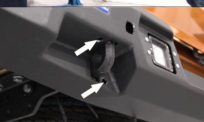
21. Fix bumper body in the area of towing hooks using screws M10x30 (14) and washers M10x20(16). Do not tighten yet.
