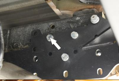
11. Mount bracket (2) on inside nut M10 (5) using bolt M10x40 (10) and washer M10x20 (16). Do not tighten yet.
