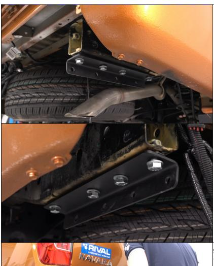
8. Mount reinforcements (6 and 7) on vehicle frame from left and right side using bolts M12x1,25x40 and washers M12x24 (17). Do not tighten yet.
