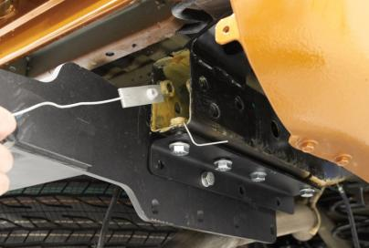
12. Mount inside nut M10(5) into the vehicle frame from the right side.
