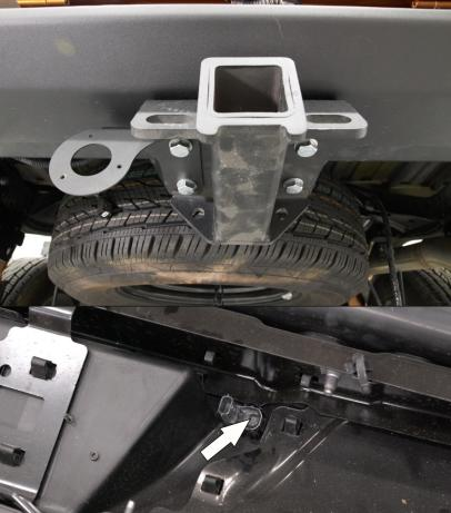
24. Mount tow bar bracket on vehicle using bolts M12x40 (11) and washers M12x24 (17). Tighten all screws.
