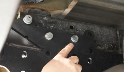
14. Mount bracket (2) from left side of vehicle into OE hole using bolt M12x1,25x40(12) and washer M12x24(17). Do not tighten yet.
