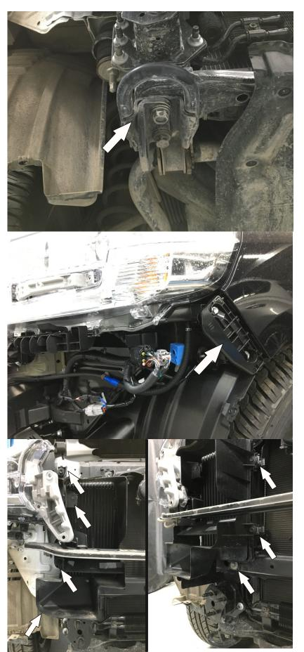
17. Unscrew 2 bolts and remove towing eye on each side.
