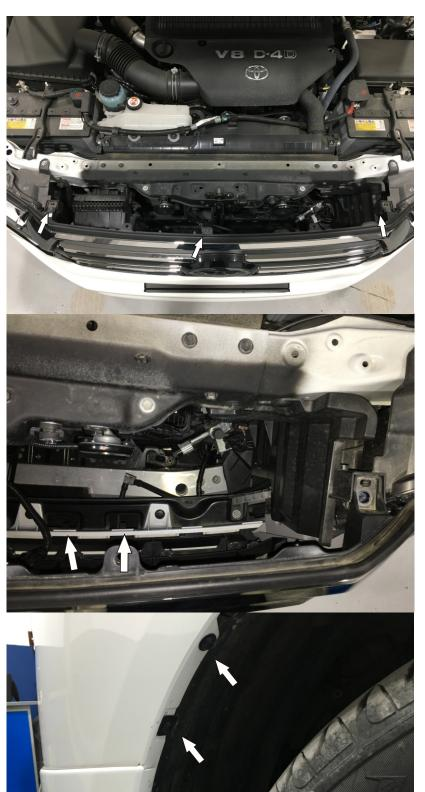
5. Remove upper grille retaining screws.
