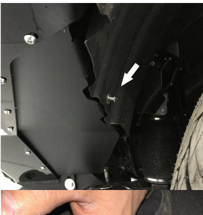
28. Mark and drill 3 holes in plastic fender in accordance with holes in flap (5, 6) on each side of the vehicle. Fix flaps (5, 6) and fenders using screws M6x20 (B).
