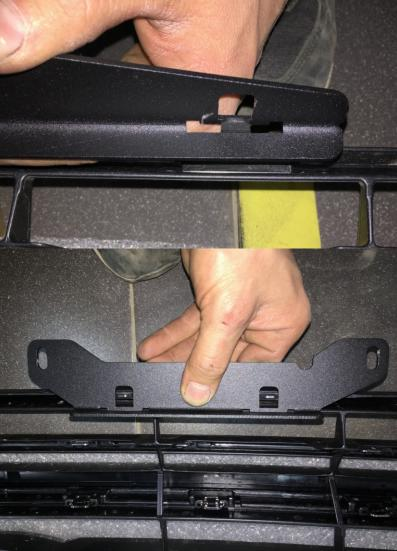
29. Instal left (8) and right grille brackets (9) on the grille.
