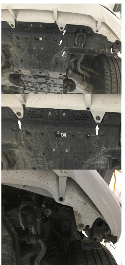
8. Remove lower bumper retaining screws.
