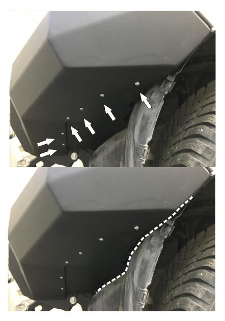
26. Install flaps (5, 6) using screws M6x20 (B) onto the bumper facing (1) on each side.
