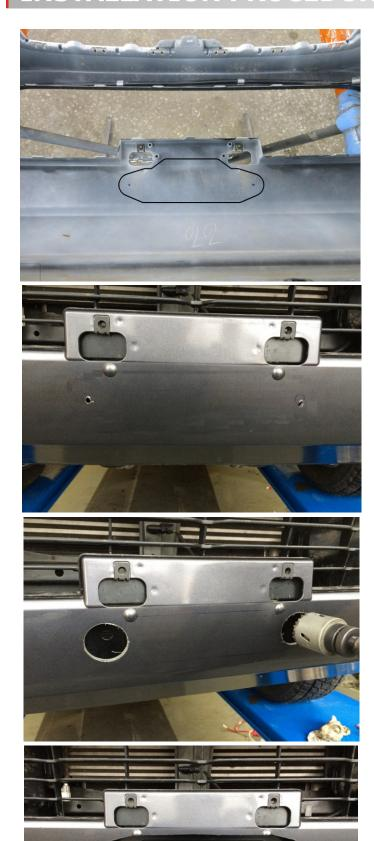
15. Temporarily place plastic bumper back to its place to mark cutting line for the fairlead
