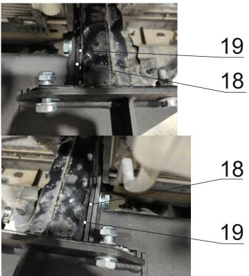
12. Install the spacers (18) as shown in the photo. In case of gaps between the beams of the car frame and the winch bracket, after installing the spacers (18), install the adjustment spacers (19) in the places indicated in the photo.
