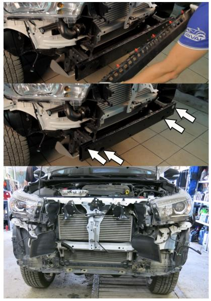
9. Remove 4 bolts and dismount front bracket as shown.
