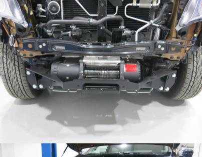
30. Install the winch bracket onto the vehicle. See paragraph 25.
