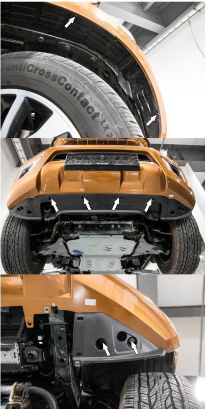
8. Unscrew 2 self-tapping screws of the bumper clamp in arches on the left and right.
