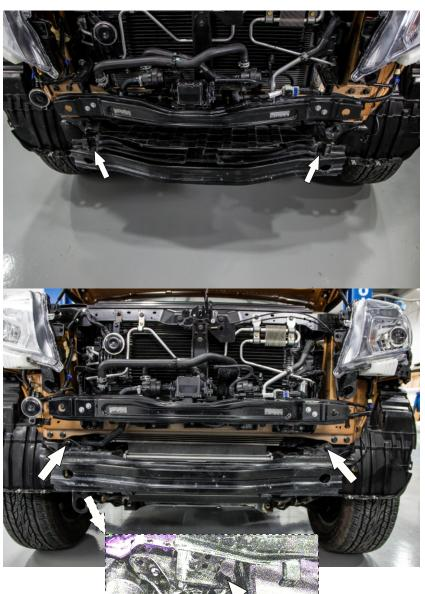
18. Remove the air intake clips. Dismantle the air intake.
