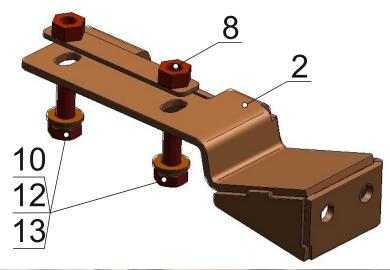
22. Install left frame booster (pos. 2) onto the vehicle frame and secure it to embedded part M12 (pos. 8), bolts M12x1,25x40 (pos. 10) and washers (pos. 12). Do not tighten screw joints.
