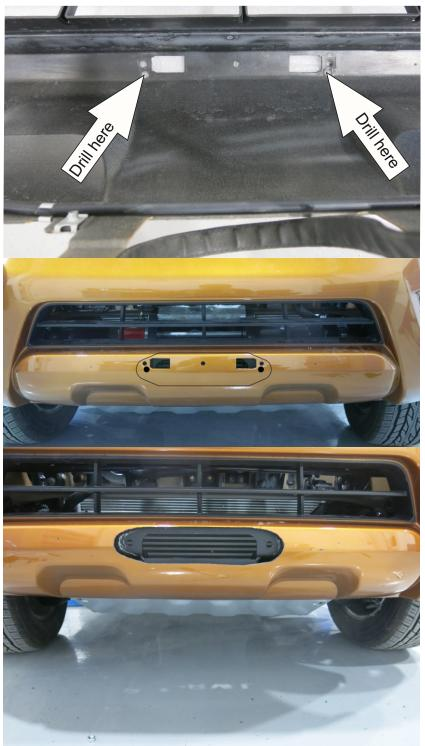
26. Temporarily install standard bumper for pad eye hole spacing. Mark the hole for pad eye fasteners on the inside of the bumper along the winch bracket.
