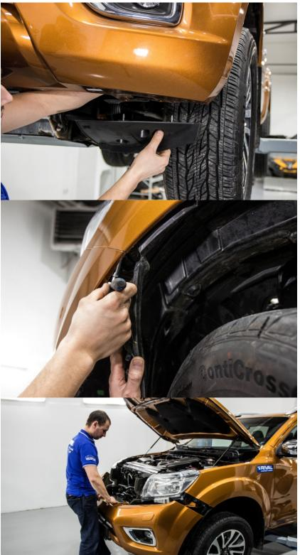
11. On the bumper inside unscrew 2 retaining nuts of the bumper skirt side and dismantle the bumper skirt side.
