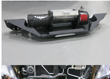
29. Remove the winch bracket from the vehicle, install the winch and pad eye onto the bracket and secure with bolts from the set of winch and pad eye.
