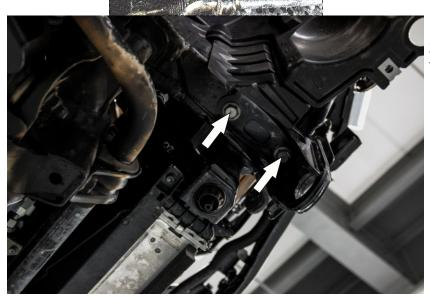
20. Unscrew 2 tension bolts of standard towing eye. Dismantle the towing eye.
