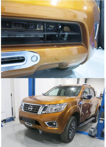
33. Install number frame and radiator grille onto the vehicle.
