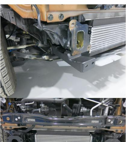
23. Install right frame booster (pos. 3) onto the vehicle frame, secure with standard bolts with installation of standard towing eye. Do not tighten screw joints.
